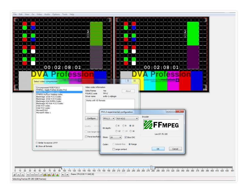
Encodes RAW audio-visual data (DPX/TIFF) into a losslessly compressed file (no more unplayable TAR!)
